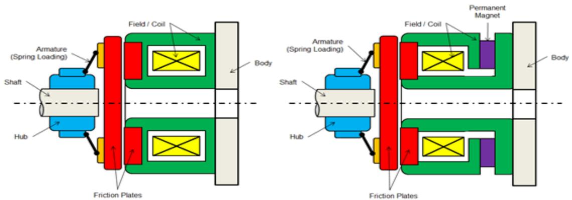
**Figure 1:- Electromagnetic Braking System.**
