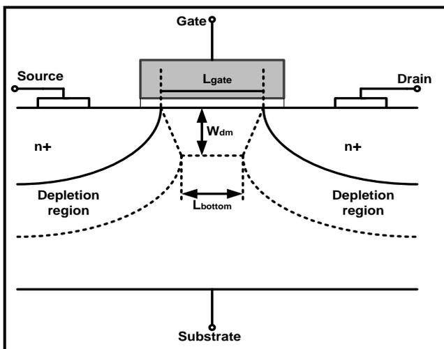
Fig.3: NMOS transistor of the depletion regions in short channel device
