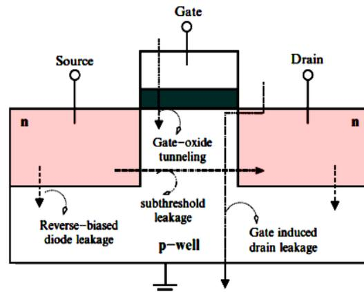
Fig. 2: Components of Leakage Power Dissipation [2]
