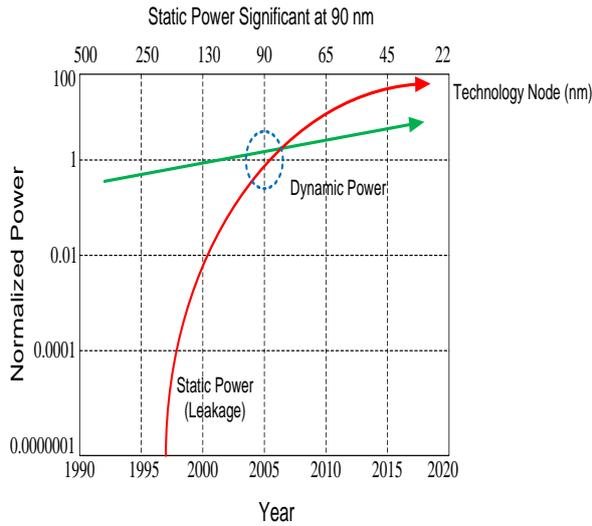
Fig.1. Enchantment of leakage power with scaling of technology in Intel Chip.
