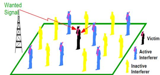
Fig. 2: Framework of Victim-Interferer model for Monte Carlo simulation
