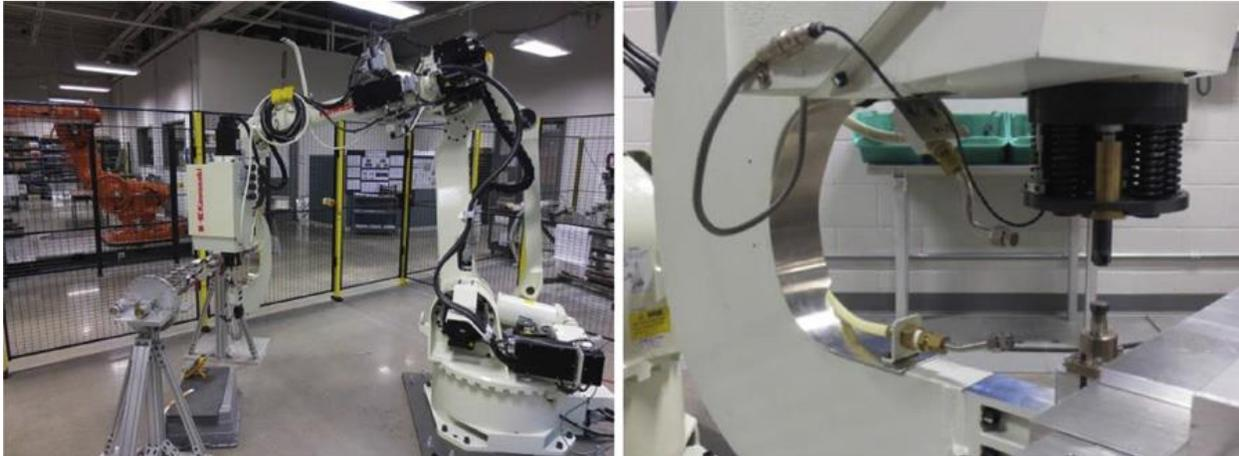
Fig. 2. Kawasaki Robot for FSW
